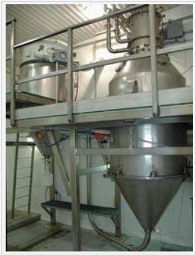
Pilot-scale pulse combustion spray
